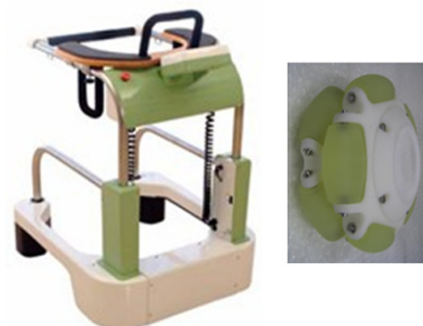
Figure 1. Omni-directional walkers and one of its omni-directional wheels
