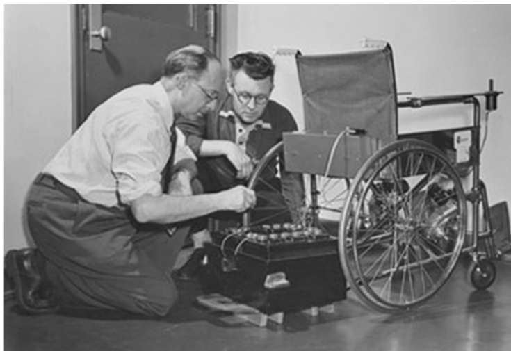
Figure 1. George Klein works on the first practical powered wheelchair at the NRC (Image property of National Research Council of Canada Archives)
