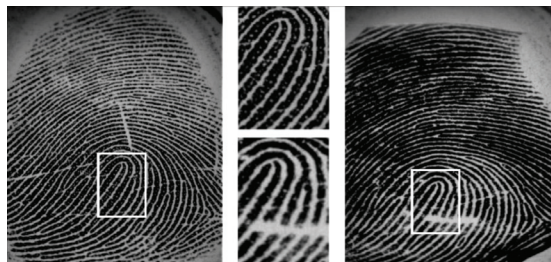
Figure 1. An example of live and fake fingerprint images (left and right side, respectively) corresponding to the same subject. At the center, we zoomed on the rectangle pointed out in both images, in order to point out differences mainly due to the fabrication process of the fake fingerprint.
