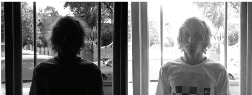
Figure 1. Images captured with a conventional camera using different exposure settings and global gain adjustments. Left) short exposure time which lets the bright background be seen but misses the darker foreground. Right) long exposure time which over-exposes the background saturating it and resulting in a loss of information, however more foreground detail is present. Traditionally camera operators had to decide which one of these modes they would operate in due to the limitations of the image capturing and processing technology.
