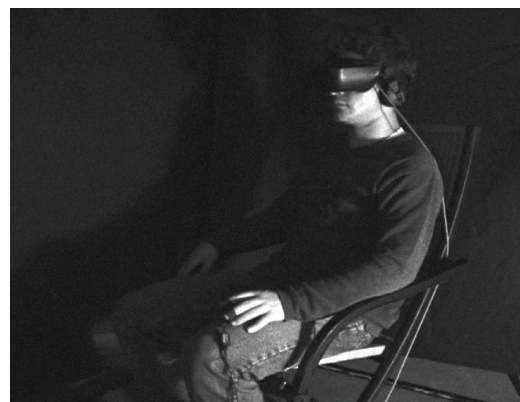
Figure 1. The Meditation Chamber. Users wear a head-mounted display (HMD) that provides them with stereoscopic imagery and sound. Interaction primarily occurs as users strive to manipulate their physiological states via biofeedback. Biometric sensors are attached to two fingers with Velcro; these sensors tracked galvanic skin response and heart rate. A flexible chest band tracked respiration.
