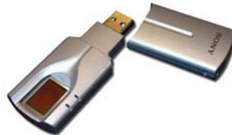
Figure 5. Sony®'s Puppy® Fingerprint Identity Token by Corp 5
