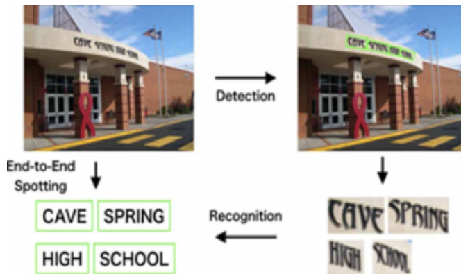
Figure 1. Diagrammatic representation of the process of detecting and recognising text in a picture
