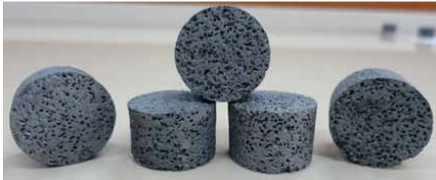
Figure 1. Steel foam specimens having different porosities (Beköz, 2011)
