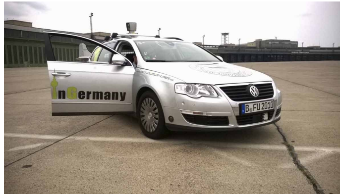
Figure 1. The autonomous car “MadeInGermany” used in the AutoNOMOS Project. Source: Rotter (2014).
