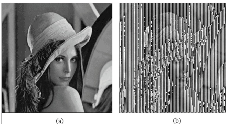
Figure 1. The image is encrypted by DES directly. (a) Original image, and (b) Encrypted image
