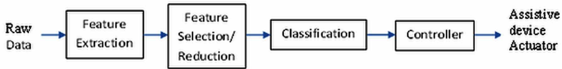
Figure 1. Block diagram of pattern recognition based control of assistive device
