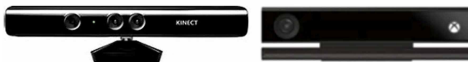
Figure 1. Two versions of Microsoft Kinect sensors. On the left is the Kinect v1. On the right is the Kinect v2.
