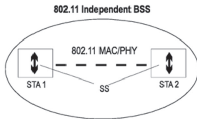
Figure 1. IEEE 802.11 ad-hoc network
